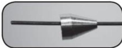
❷ Unscrew cap from the base of the Conduit Rat™; separate the Conduit Rat™ into point and base. Next, slide base onto the end of the fish tape.
