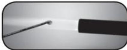
❸ Apply heat to end of fish tape and bend tip of fish tape at 3/16" using pliers, as shown. Allow tape to completely cool.
